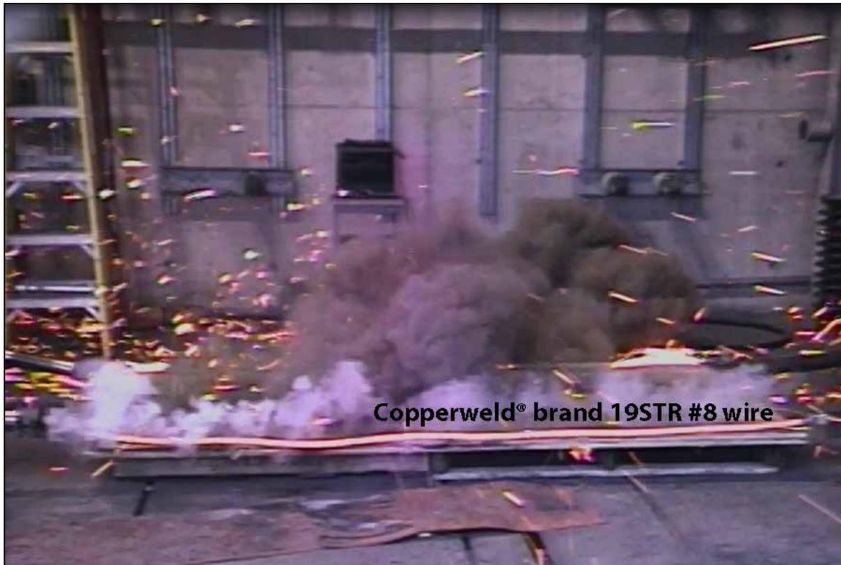
**Figure 4. One article (conductor) left; At time: ~30 cycles (~500 ms), Copperweld® brand 19STR. #8 wire remains intact.**
